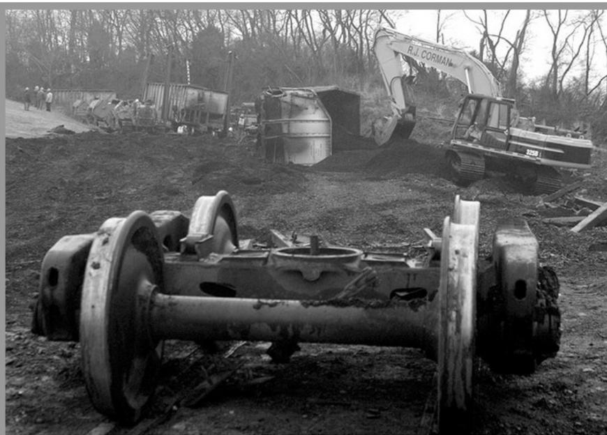
A damaged truck from a loaded coal hopper bears mute testimony to the damage done in a derailment of a CSX unit coal train on the Pee Vee Spur just west of Madisonville. One locomotive and 8 cars were involved in the mishap which took place the evening of February 8. *digital photo by Jim*
